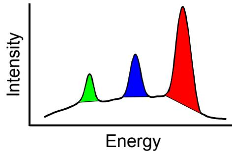
Figure 2: LEIS spectrum for the experiment in fig. 1. The energy after a collision with a heavy atom (red) is high whereas the energy after a collision with a light atom (green) is low.
