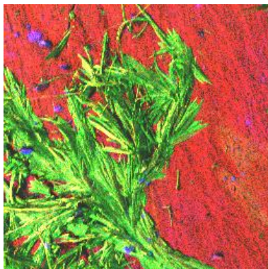
Figure 3: RGB colour overlay of the PP matrix (red), the phosphate antioxidant Ultrinox 626 (green) and the release agent Li-Stearate, blue). Field of View: 500 x 500 \mu\text{m}^2 .
